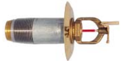
QUICK RESPONSE DRY NON-ADJUSTABLE HORIZONTAL SIDEWALL
